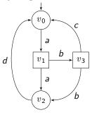
A two-player turn-based finite arena  $\mathcal{A} = (V_{\square}, V_{\square}, E)$  with no deadlock.
